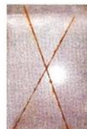
Steel Guard Coated followed by single coat of Epoxy Paint after 1200 Hours in Salt Spray Machine as per ASTM-B-117.
